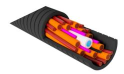
The division of the power cables into several small individual ones and the stranding of these individual wires results in a high flexibility of the charging cable. In the center of the cable is the supply line for the coolant, which flows back between the individual, insulated cores. This provides excellent cooling and high flexibility of the cable. In combination with the paXos charging plug, a particularly powerful and convenient charging system is provided.
