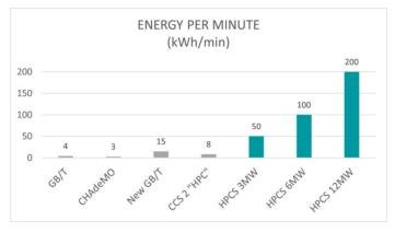
In the future, the classic "pin & socket" connector will be one of the limiting factors within the charging infrastructure. The increase in the size of the connectors leads proportionally to higher plug-in forces, which have a negative impact on operability. With the "Cool-Load Megawatt" from paXos, which has ring-shaped contact surfaces, the charging power can be adapted to future requirements simply by scaling the connector diameter. In this way, outputs of up to 40MW are possible.
