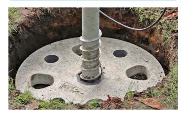
The paXos Rapid Foundation System (RFS) imitates the tree root principle. Central taproots absorb high tensile forces and surface roots absorb the bending and shear forces. The RFS therefore combines an earth screw, which absorbs the tensile forces, with a rigid prefabricated concrete slab, which is placed just below the turf and absorbs the bending and shear forces.
